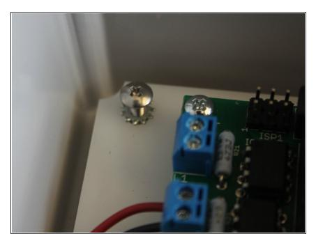
Mount Plate into enclosure base with 4 to 6 screws.
