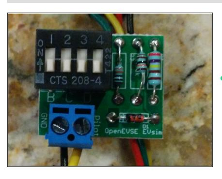
EVSE states can be tested with a few resistors and a diode, and EV Simulator or an EVSE Tester. After a successful Power on Self Test OpenEVSE should enter State A - Ready and the LED/LCD should be Green.
