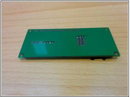
• Solder the 3&4 pin right angle headers to the OpenEVSE LCD logic board.
