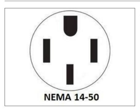
NEMA 14-50 commonly called an "RV outlet" is recommended to charge your vehicle Level 2 at up to 40A.
