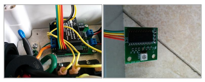
Connect 4 pin LED cable to the OpenEVSE board.
